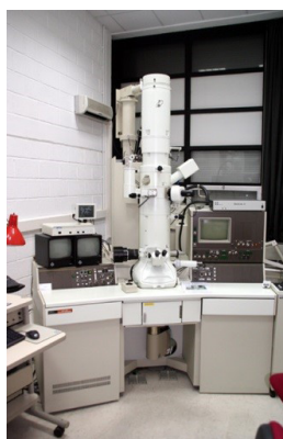
TEM with a system of filtered imaging (GIF) and beam scanning (STEM)
