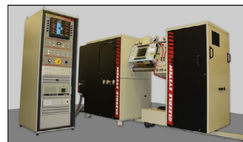
Gleeble 3800 for high pressure physics simulations (20t) and thermomechanical characterization (© Gleeble)
